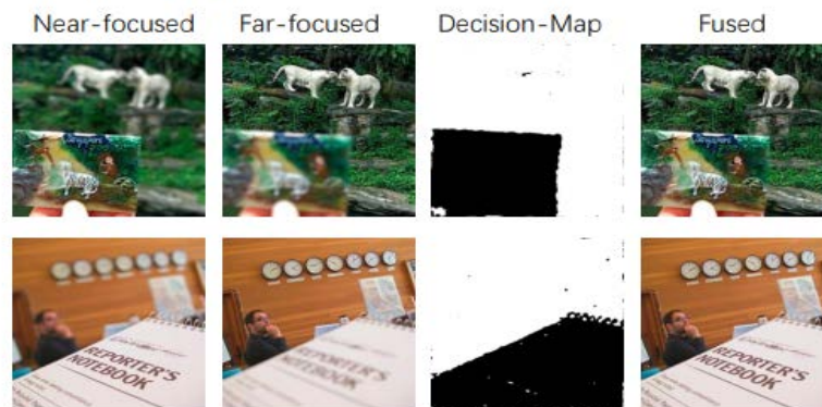
Fig. 1. Test results of PATN on the Lytro dataset. From left to right are: Near-focused, Far-focused, Decision-Map, and Fused images.
